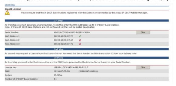
The red cross means that the IP Base Station with that MAC address has not tried to connect with the ADMM.
